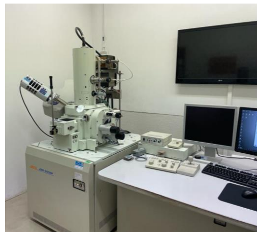
Figura 51 – MEV Zeiss DSM 962 (Electron gun: W filament, Accelerating voltage: 1- 20keV, “Out-lens” detectors, Oxford INCAx-act LN2-free Analytical 10 [mmX] Silicon Drift Detector with PentaFET precision, resolution of 125eV, JEOL JSM 6500F + EDS Oxford.X – Max; Fabricante – Zeiss.
