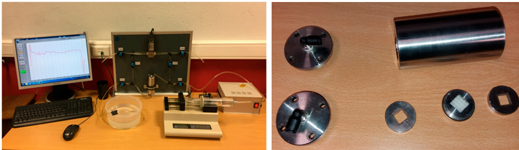
Figure 2. Experimental apparatus for the permeability tests (left: overview; right: permeability chamber parts).
