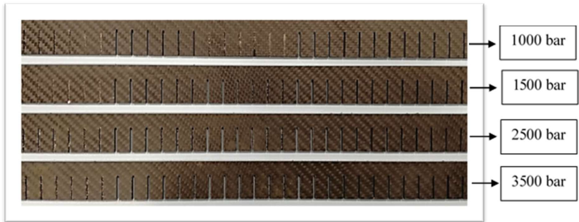
Figure 25. Samples obtained to realize water jet process
