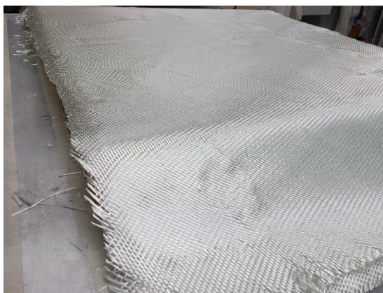
71. Image Lay-up sandwich panel
