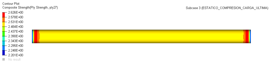
50. Table Laminate type. Ultimate load to compression. Reserve factors of tube fabrics. Own elaboration
