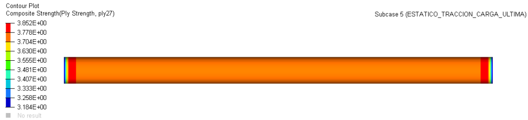
54. Image Ultimate load to traction. Reserve factor in critical fabric (Ply 27). Own elaboration
