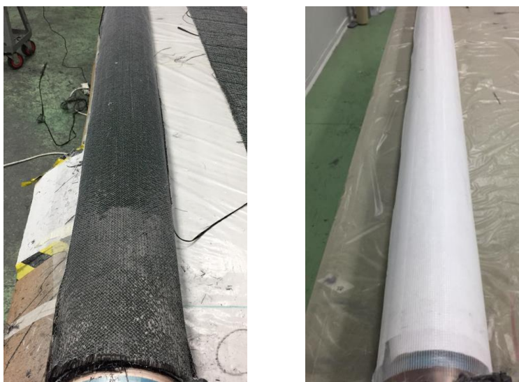
63 Image. Carbon lamination and final peel ply and infusion mesh. Own elaboration
