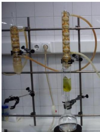
Figura 9 - Extrator de Soxhlet.
