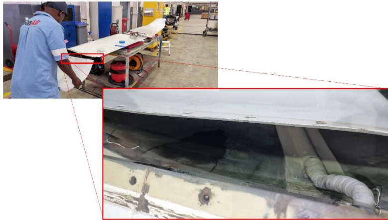
Figure 26 – Inside the lowered part of the Horizontal Stabiliser of AW189 under Maintenance
