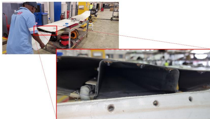
Figure 27 – Inside the Upper part of the Horizontal stabiliser of AW189 under Maintenance
