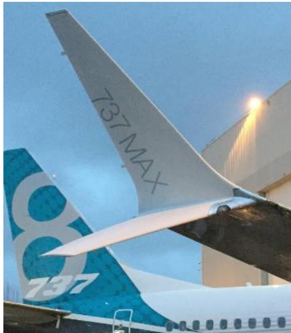
**Figura 1** – *Split winglet* do B-737 MAX (Simpleflying, 2023).
