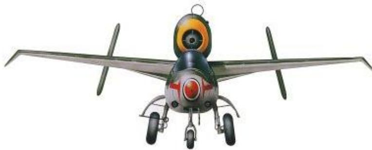
**Figura 3** – Heinkel He 162 equipado com “*Hoerner tips*” (Aerodyn, 2001).
