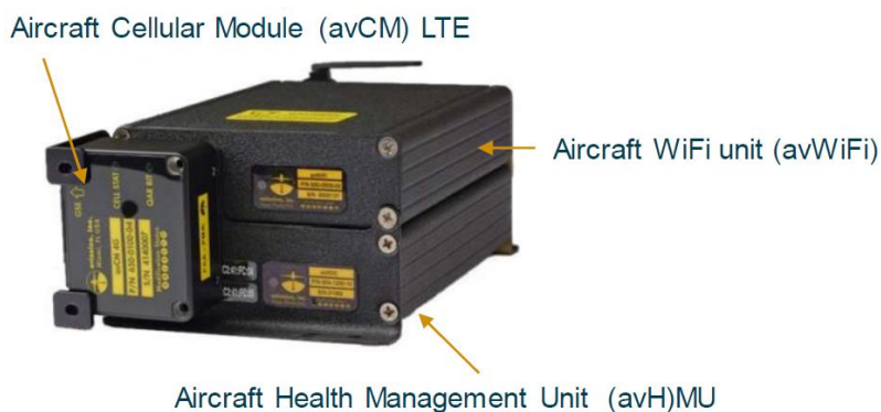
Figure 6- AHMU and Surrounding Components
