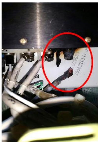
Electrical lug and WHTC stud damaged
