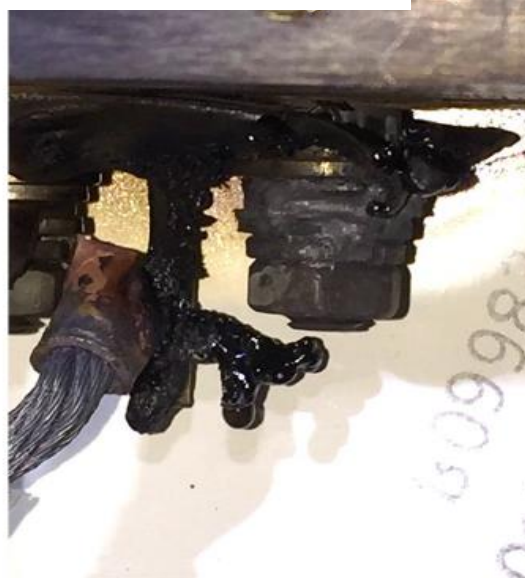
Electrical lug and WHTC stud damaged
